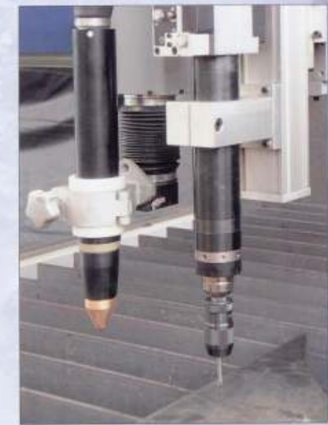
Option Additional drilling unit on the torch carrier (ZINSER 2315-N and ZINSER 2325-N)
